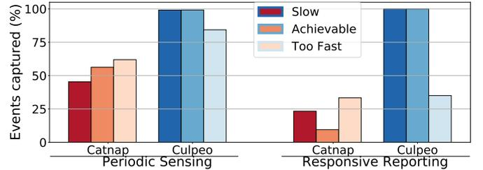
**Fig. 13:** Culpeo has nearly ideal event capture for achievable event rates. Catnap misses events because its  $V^{\text{safe}}$  predictions are wrong. CatNap discharges the capacitor too low while performing background work in between events, so the more time between events (i.e. the slower the event arrival rate) the more likely the task is to fail.
