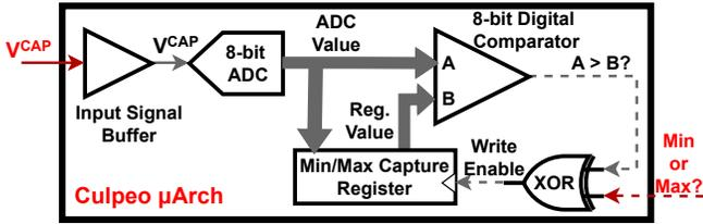
**Fig. 9:** The Culpeo- $\mu$ Arch is a low overhead design that uses an 8-bit ADC, a comparator and a single register to track capacitor voltage for Culpeo-R. Red arrows indicate inputs, solid arrows are analog signals, dashed arrows are boolean and wide arrows are 8-bit buses.
