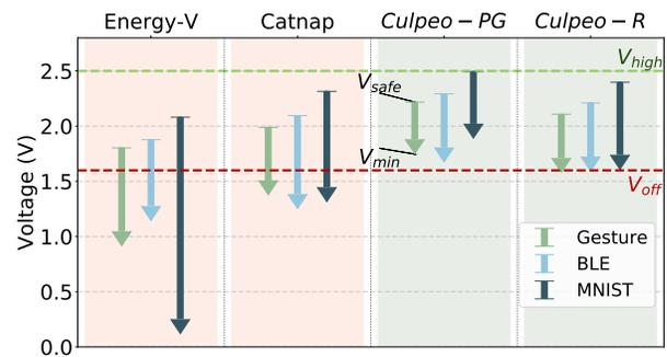
**Fig. 11:** Culpeo-R and Culpeo-PG's  $V^{\text{safe}}$  values (arrow tops) complete with  $V^{\text{min}}$  (arrow points) above  $V^{\text{off}}$  for tests on three real peripherals. The graph shows that Energy and CatNap  $V^{\text{safe}}$  estimates are unsafe, because they cause the device to turn off unexpectedly.
