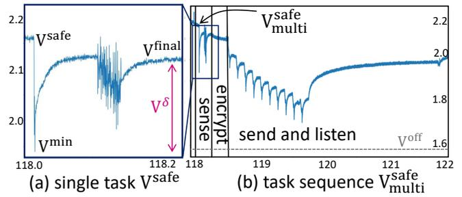
**Fig. 8:** A measured  $V^{\text{cap}}$  trace over a single (a) and multiple (b) tasks:  $V^{\text{safe}}$  guarantees that a task will complete, but the  $V^{\delta}$  parameter is required to calculate  $V^{\text{safe}}_{\text{multi}}$ , a safe voltage for a sequence of tasks.
