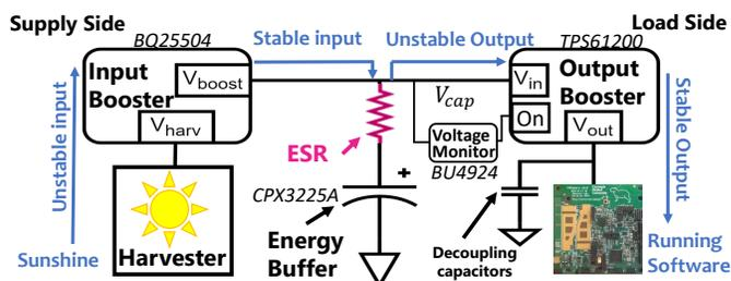
**Fig. 2:** An Annotated energy-harvesting power system schematic. An EHD harvests energy into a (super)capacitor and uses the energy to run software tasks. Input and output boosters regulate voltage to the energy buffer and the load, respectively.
