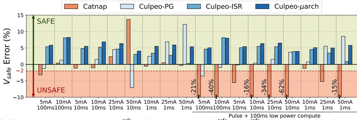
**Fig. 10:** This graph shows the error between  $V^{\text{safe}}$  predictions and the actual  $V^{\text{safe}}$ . The  $V^{\text{safe}}$  estimates produced by Catnap and other energy-based methods produce radically incorrect estimates. All Culpeo variants produce safe ( $> 0$ ) and performant ( $< 10\%$  error) estimates.
