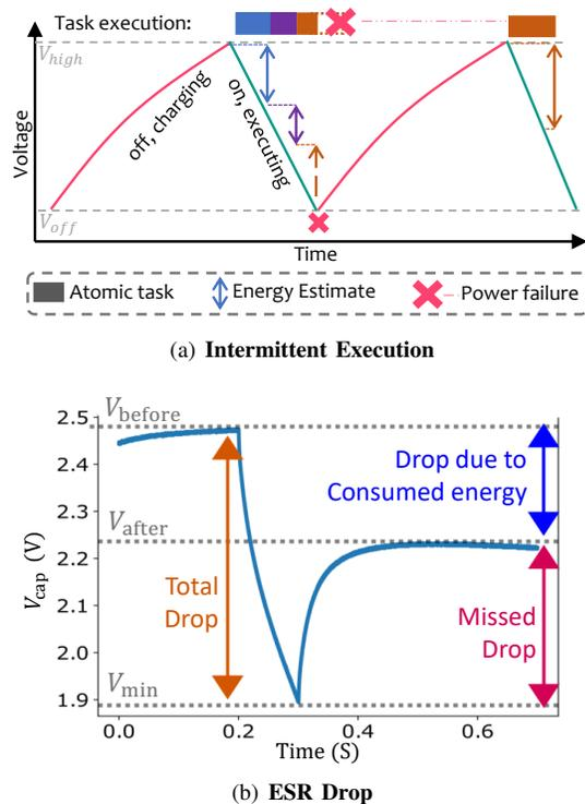
**Fig. 1:** 1(a) shows an intermittent execution trace. Consuming energy lowers the device’s voltage level; if it drops below  $V_{off}$ , the device powers off. Software atomic tasks must re-execute from the beginning after such a power failure. 1(b) shows voltage drop and rebound due to ESR on a real trace, which causes the problem addressed by this work. Considering only energy consumption misses this key voltage drop, leading to incorrect charge management.
